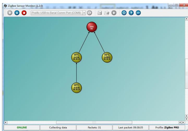
As the picture shows, the  $01^{\circ}\text{C}$  means the count of getting topology of network, "0x3A94" means the short address of the module, "09:40:11" means the time of getting topology of network.
