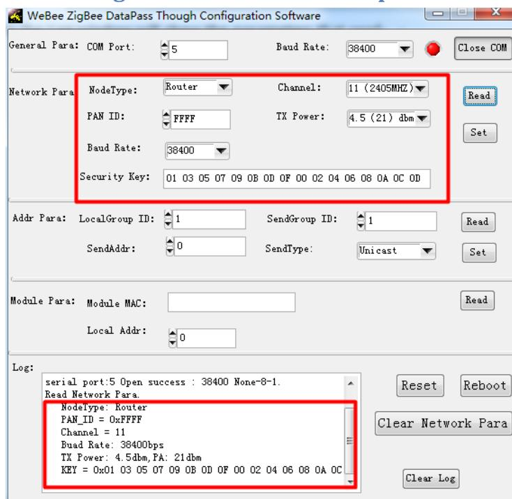
**4.5 Set parameters. Fill the ZigBee network parameters, then click the “Set” button. If successful, the log window will show the value that has set.**
