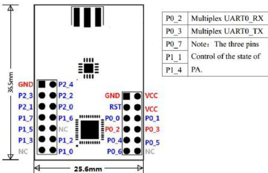
If the customer use Z-002 ZigBee transparent transmission module , you only need to focus on the function and use of the following pin, it can directly interact with external serial devices, to implement ZigBee wireless communication.
